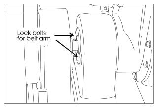
Figure 2: Lock bolts for belt arm
