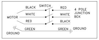
Figure 31: Schematic diagram for 3-phase motor.
