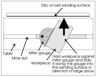
Figure 5: Use of the miter system
