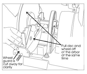
Figure 13: Removing the guard and drive disc, together.
