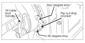
Figure 21: Locations of stop lugs and stop bracket for zero and 45° table positions.
