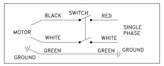
Figure 30: Schematic diagram for single phase motor.
