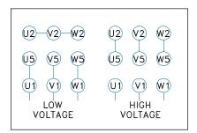
Figure 33: Motor connection diagram for 3-phase motor.
