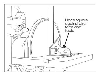
Figure 15: Using a square to check the disc table scale.
