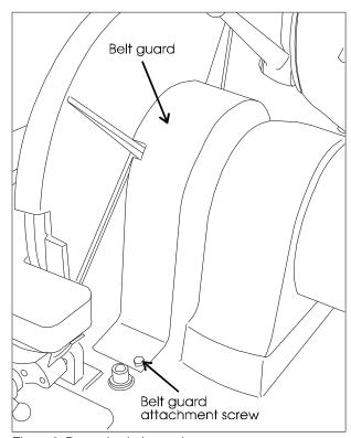
Figure 9: Removing belt guard
