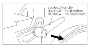
Figure 1: Locking handle for belt table
