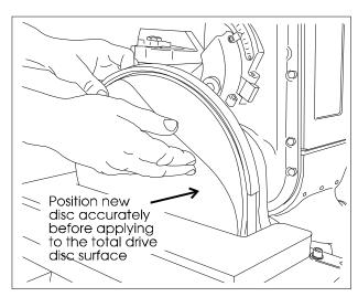
Figure 8: Installing new abrasive disc
