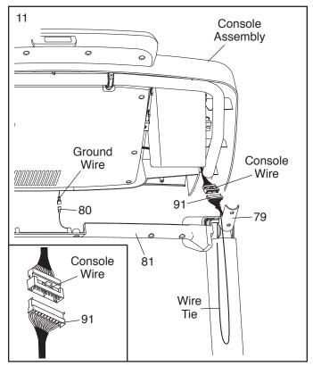
12. Set the console assembly on the Left and Right Handrails (79, 83). **Make sure that no wires are pinched.** Insert the excess Upright Wire (91) behind the Console Frame (101).
