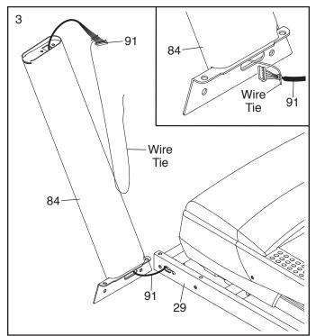
4. Hold the Left Upright (84) against the Base (29). Be careful not to pinch the wires. If necessary, position the base ground wire (A) in the hole in the side of the Left Upright. Insert two 3/8" x 2 3/4" Screws (22) and two 3/8" x 1 1/4" Screws (3) with two 3/8" Star Washers (10) into the Left Upright.
